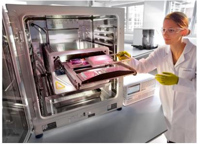
Using a microscope and imager that stays with the cells in an incubator
